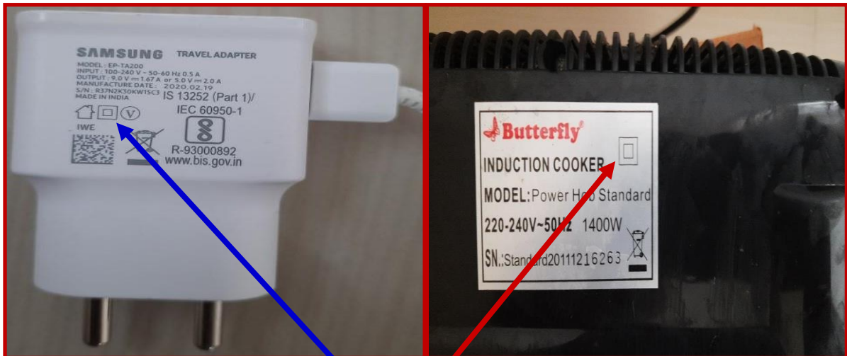
Class II Equipment Symbol on i) Mobile Charger and ii) Induction Stove
